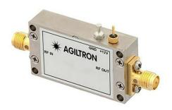
This is high gain low noise amplifier with 27dB gain in the frequency of 1-18GHz. The DC power requirement is +5V/100mA. The module is with SMA connector. We can provide all kinds of coaxial low noise amplifiers, with frequency from 0.01-67GHz, gain from 20 to 60dB, Pout from +5 to +27dBm, and connectors from SMA to 1.85mm.
